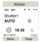
Room allocation (optional) Function bar: ↔ = Bidirectional → = Unidirectional Channel number or name of the channel Operating mode, status symbol
